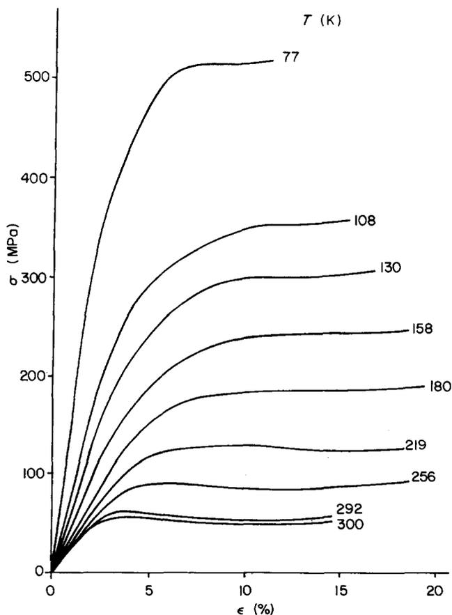
**Figure 3** Stress-strain curves for EPO 40/60
