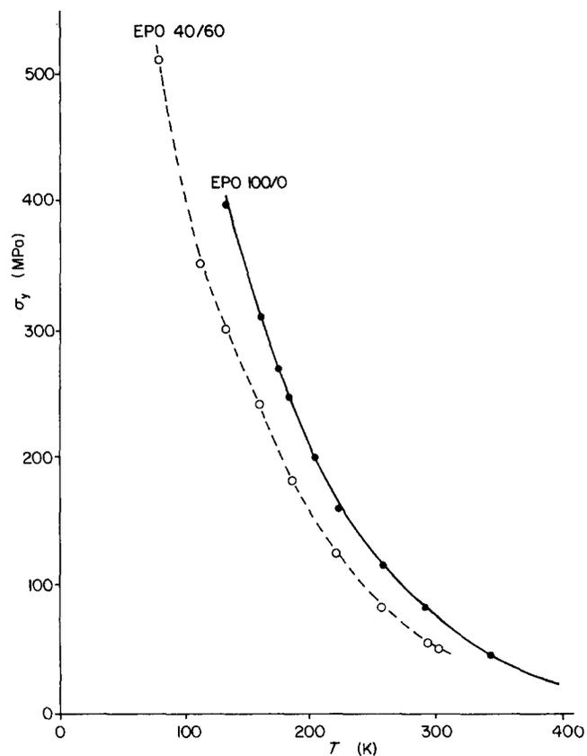
Figure 5 The temperature dependence of the yield stress  $\sigma_y$
