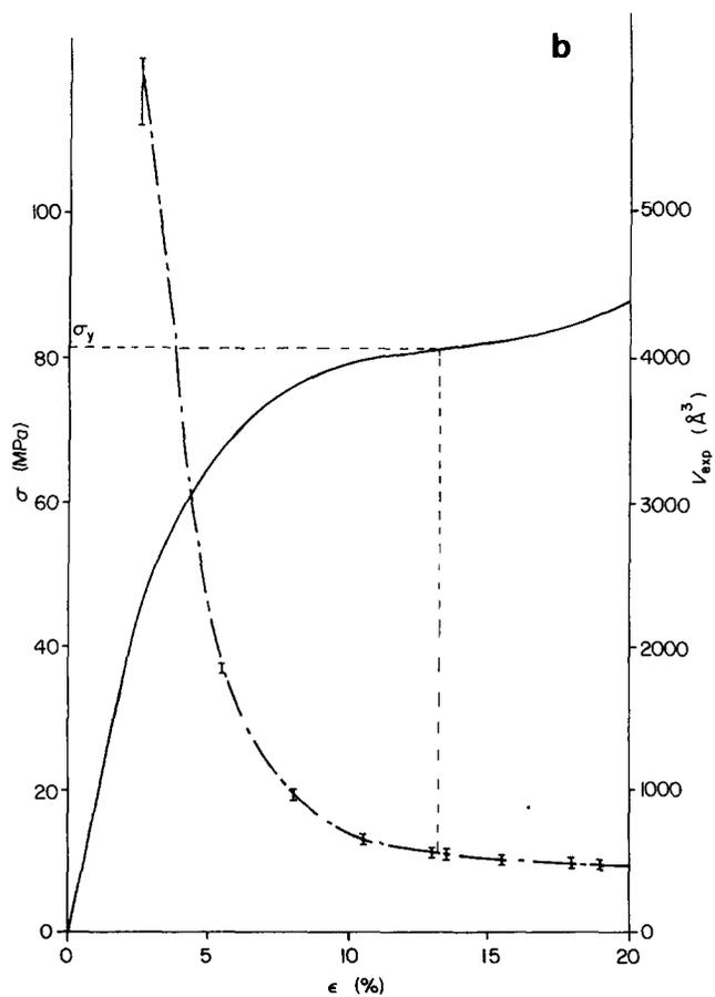
Figure 4 Definition of the yield stress  $\sigma_y$ : (a) EPO 100/0 network; (b) EPO 40/60 network ( $T = 20^\circ\text{C}$  for both)
