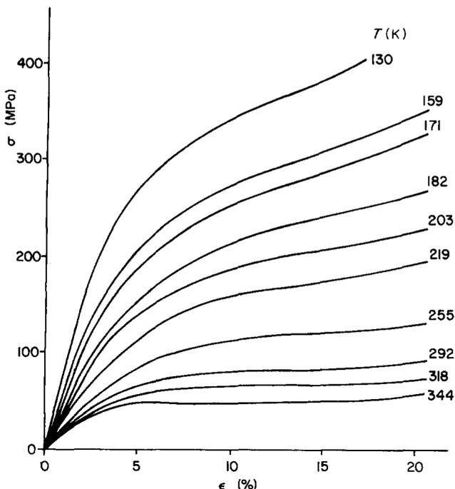
**Figure 2** Stress-strain curves for EPO 100/0
